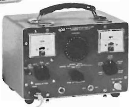
Singer Metrics "Gertsch" FM-9 combines the functions of direct-reading frequency meter, FM deviation meter, and accurate signal generator. Its accuracy is 0.0002%. ($1595)
