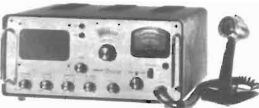
Tram "Titan" CB base station uses frequency synthesis, audio compression, mechanical filter in receiver, multi-function meter. ($434)
