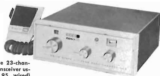
The e.c.i. "Courier TR-23S" is a compact, silicon-transistor CB transceiver measuring only 5 3/4" x 1 7/8" x 6 1/4" deep. ($169)
